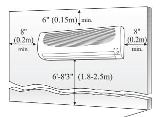
Fig. 2 — Indoor Unit Clearances
